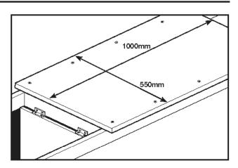
2 IMPORTANT: The bar side of the roller bar bracket MUST be nearest to the hatch. Fix the bracket centrally using four 40mm screws (B4) study diagram closely. The edge of the bracket must be positioned right up to the edge of the hatch opening.
