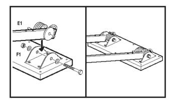
With the spring housing assembly in line with the ladder, fix it in position using six 40mm screws (F2).
