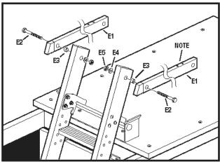
Attach the power arms (E1) to the spring housing assembly (F1) with the loop end of the springs pointing away from the hatch. Remove the bolts holding the springs and insert the power arm in-between the plastic spacers then refit. Ensure the spacers locate in the power arm holes.
