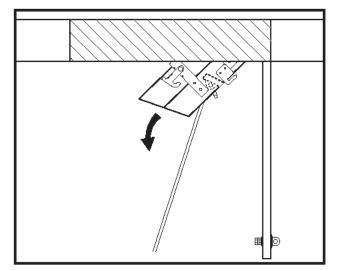
Care is needed when fully extending the ladder. Release the bottom locking catch 'A' and slide the front frame downwards until the top stops reach the upper guide brackets. Lower the ladder until the feet rest firmly on the floor. Engage locking catch 'B'. Ensure location plates are correctly located on the roller bar.
